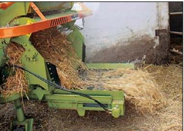
*It is specially suitable to distribute straw in standing litters and sleeping berths, as it allows to unload the cut product far from the machine, at a variable distance. In closed position, the conveyor is comprised in the machine overall dimensions. Its release is helped by a hydraulic cylinder. All this renders the machine easily-handled and suitable for many different situations.*
