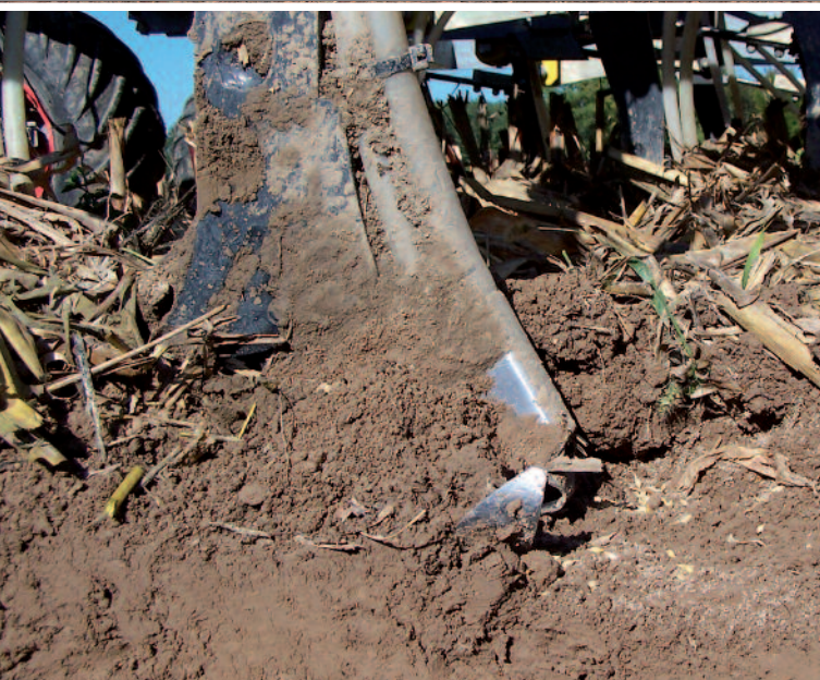
Details of opener working
