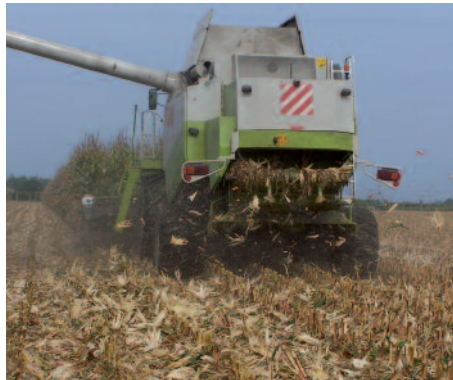
Corn harvesting with built-in stalk-chopper.
