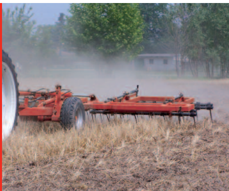
Straw Harrow on devitalized inter-row strip.
