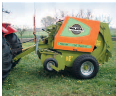
Tilting drawbar in the lowest position to allow the machine to override eventual obstacles.
